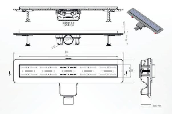
DN 50 Horizantal and vertical outlet - compatible with PVC pipe connections, blocking odor by water (285mg). The flow rate is 48 liters/min. Resistant against external chemical effects, operating temperature is between -30°C and +75°C. The and grid is made of 304 grade stainless steel.
