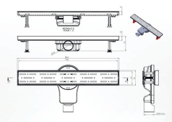
DN 50 Horizantal and vertical outlet - compatible with PVC pipe connections, blocking odor by water (285mg). The flow rate is 41 liters/min. Resistant against external chemical effects, operating temperature is between -30°C and +75°C. The and grid is made of 304 grade stainless steel.
