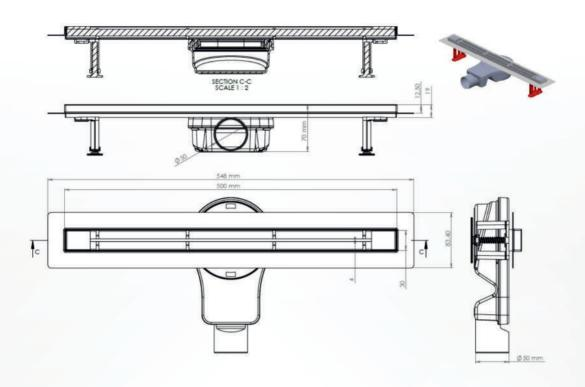
DN 50 Horizantal and vertical outlet - compatible with PVC pipe connections, blocking odor by water (285mg). The flow rate is 41 liters/min. Resistant against external chemical effects, operating temperature is between  $-30^{\circ}$ C and  $+75^{\circ}$ C. The and grid is made of 304 grade stainless steel.
