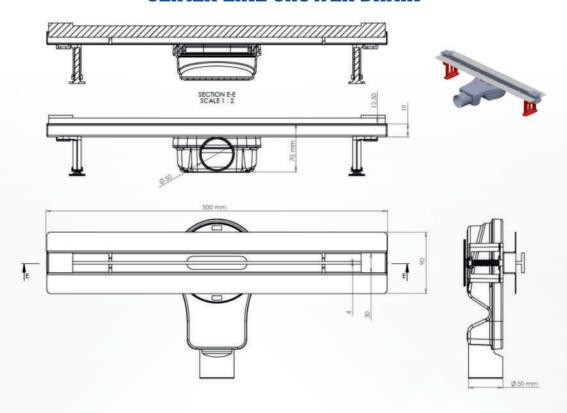
DN 50 Horizantal and vertical outlet - compatible with PVC pipe connections, blocking odor by water (285mg). The flow rate is 41 liters/min. Resistant against external chemical effects, operating temperature is between -30°C and +75°C. The and grid is made of 304 grade stainless steel.
