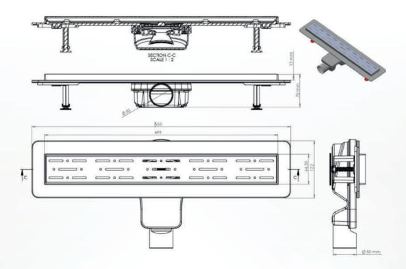
DN 50 Horizantal and vertical outlet - compatible with PVC pipe connections, blocking odor by water (285mg). The flow rate is 48 liters/min. Resistant against external chemical effects, operating temperature is between  $-30^{\circ}$ C and  $+75^{\circ}$ C. The and grid is made of 304 grade stainless steel.
