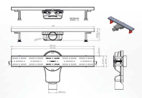
DN 50 Horizantal and vertical outlet - compatible with PVC pipe connections, blocking odor by water (285mg). The flow rate is 48 liters/min. Resistant against external chemical effects, operating temperature is between -30°C and +75°C. The and grid is made of 304 grade stainless steel.
