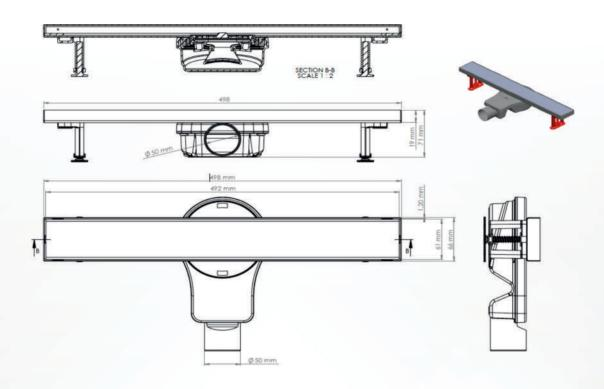
DN 50 Horizantal and vertical outlet - compatible with PVC pipe connections, blocking odor by water (285mg). The flow rate is 48 liters/min. Resistant against external chemical effects, operating temperature is between -30°C and +75°C. The and grid is made of 304 grade stainless steel.
