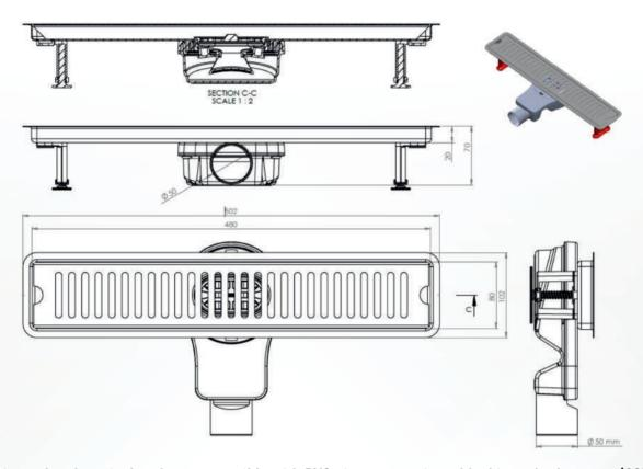
DN 50 Horizantal and vertical outlet - compatible with PVC pipe connections, blocking odor by water (285mg). The flow rate is 41 liters/min. Resistant against external chemical effects, operating temperature is between  $-30^{\circ}$ C and  $+75^{\circ}$ C. The and grid is made of 304 grade stainless steel.
